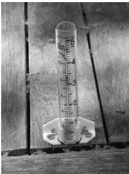
A rain gauge measures the amount of precipitation over a period of time.
